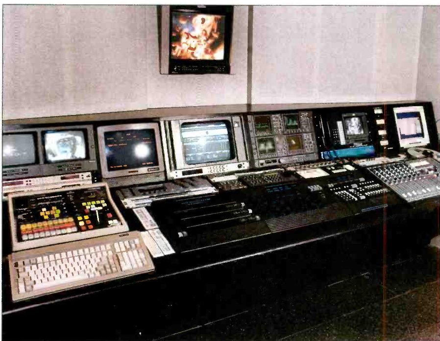
One of Post Perfect's all-digital color correction suites. Color A features a da Vinci Renaissance 8:8:8 color corrector (center console), digital and analog scopes, TLC keyboard, digital switcher and touchscreen routing switcher monitor (at far right).
