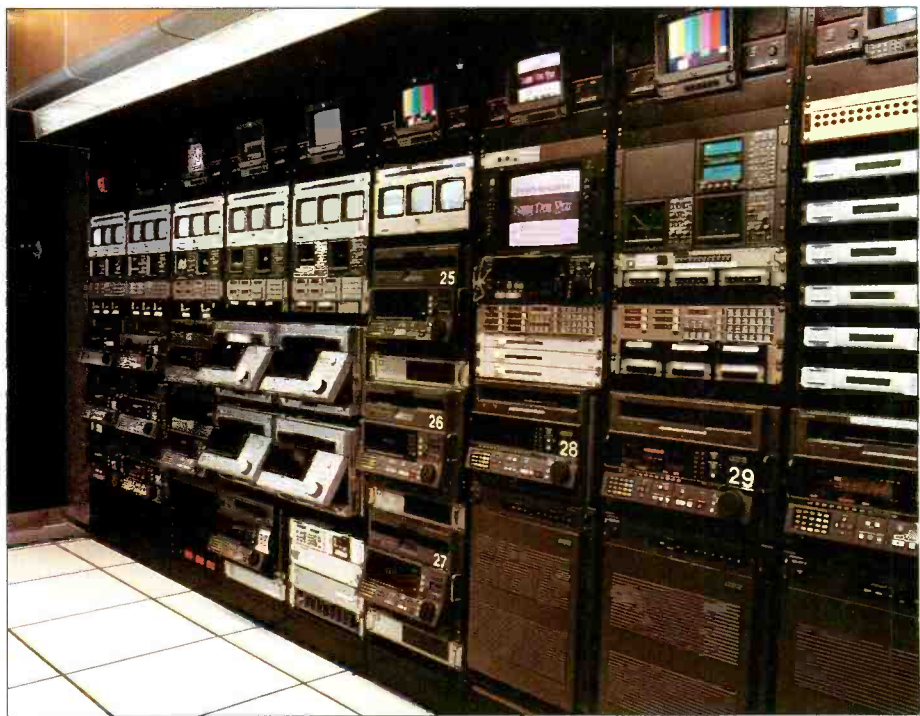
Machine Room A features (left to right) D-2, Ampex DCT and D-1 machines and Innovision encoders for the D-1 decks (at extreme right).
